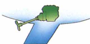
MS2B-R (R-reverse gear) Propeller shaft, 7 degree angle
